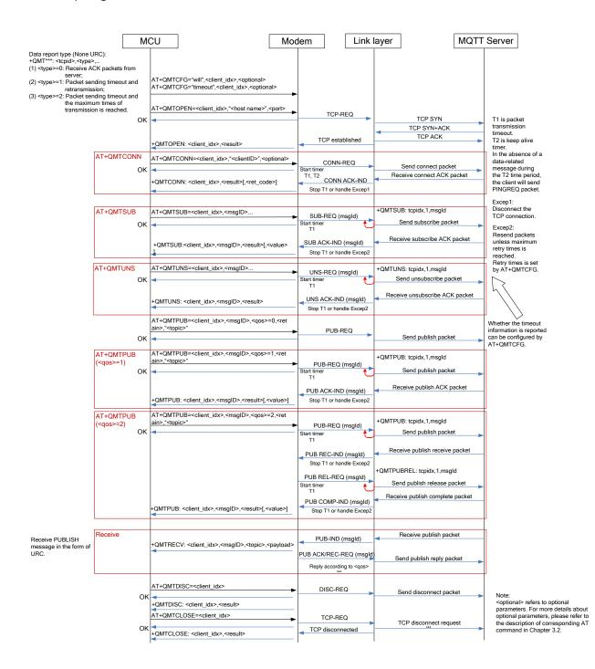
**Figure 1: MQTT Data Interaction Diagram**
